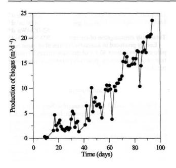
Fig. 7. Biogas production in methanogenic reactor.
