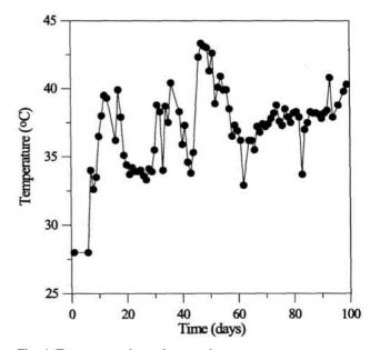
Fig. 4. Temperature in methanogenic reactor.
