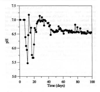
Fig. 6. pH in methanogenic reactor.
