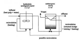
Fig. 1. Pilot-scale model of anaerobic treatment of sugar beet pulp.
