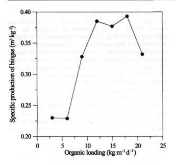
Fig. 8. Specific production of biogas at individual OLR of the methanogenic reactor.
